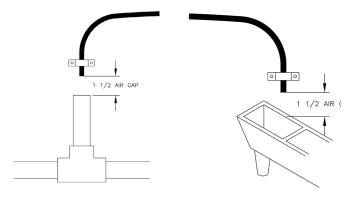
Figure 7 Required Air Gap for Drain Line
