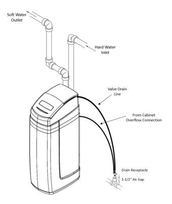
Figure 1 Plumbing with Standard Bypass
