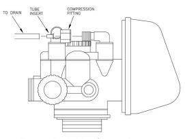
Figure 8 Drain Line Connection
