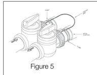
When installing sweat copper follow state and federal codes by using a lead-free solder and flux. Use a joint compound to seal threaded pipe. Some homes use the cold water pipes for an electrical ground (metal only). When finished with plumbing, a ground wire should be connected to the copper pipes to complete the ground circuit. Use two clamps and #4 copper for this.
