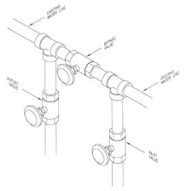
Figure 4 3-Way Bypass Plumbing
