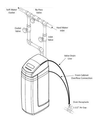
Figure 2 Plumbing with 3-Way Bypass
