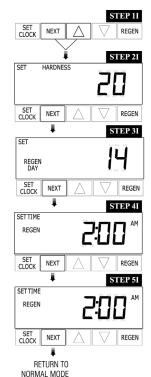
**STEP 4I –** Next Regeneration Time (hour): Set the hour of day for regeneration using the DOWN or UP arrow. AM/PM toggles after 12. The default time is 2:00 a.m. This display shows REGEN ON 0 GAL if ON 0 is selected in Step 9S or Step 7F. Press NEXT to go to step 5I. Press REGEN to return to previous step.
